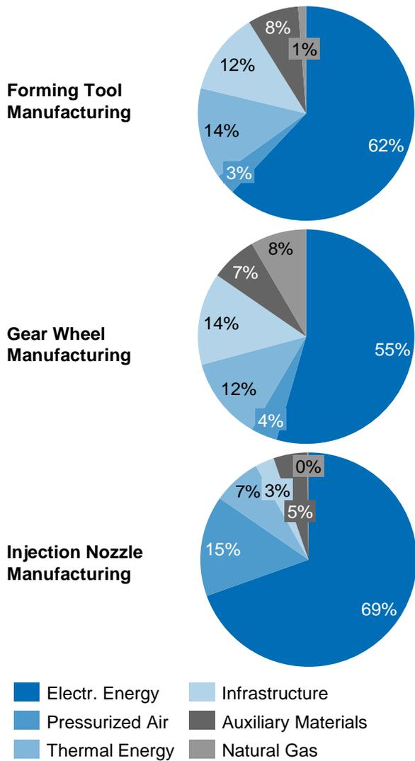
Figure 3: Shares of consumption types during manufacturing of the three case studies based on primary energy depletion (PED)
