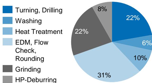
Figure 4: Shares of process consumptions during manufacturing based on primary energy depletion (PED)
