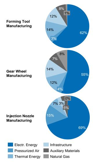
Figure 3: Shares of consumption types during manufacturing of the three case studies based on primary energy depletion (PED)
